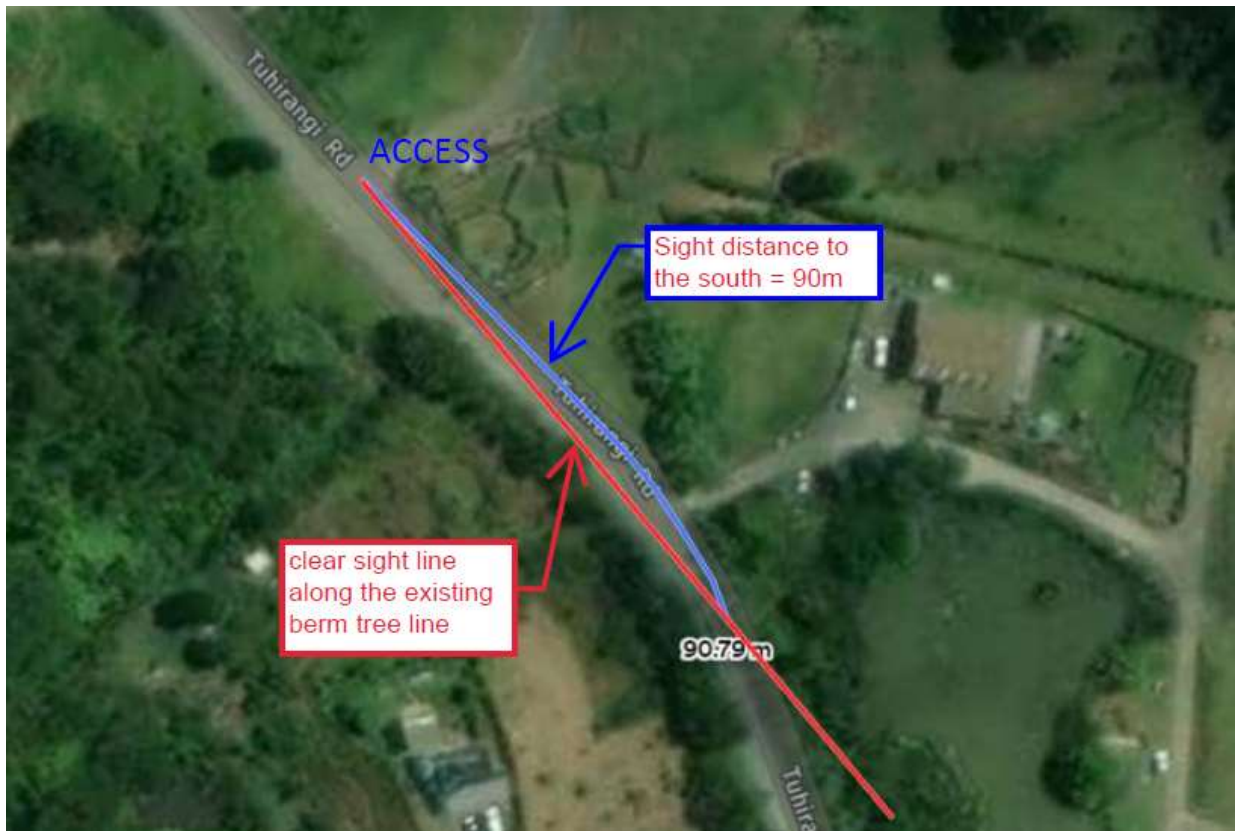
Figure 17: Desktop study sight distance to the south from site's access
